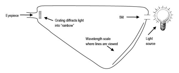
Look through the spectroscope and observe and record the colored lines (spectrum) produced by hydrogen gas. Complete the data table below and then draw the color lines in the spectrum box that follows.
