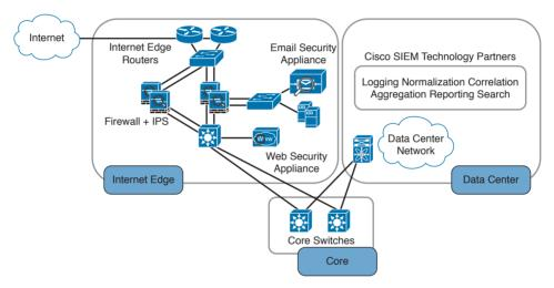
**Figure 5-12** *Typical SIEM Deployment/Key Capabilities*
