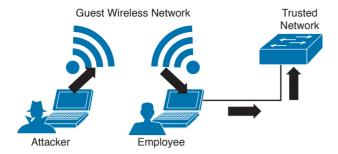
Figure 14-13 Pivoting Through a Compromised Host
