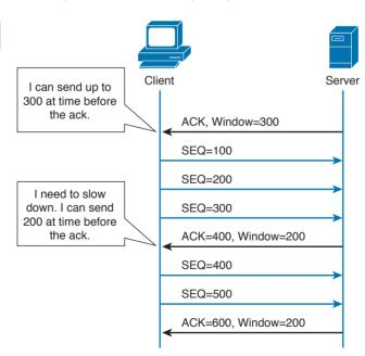
**Figure 1-86** Example of TCP Flow Control
