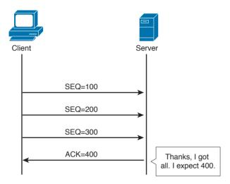
Figure 1-84 Example of TCP Acknowledgement and Sequence Numbers
