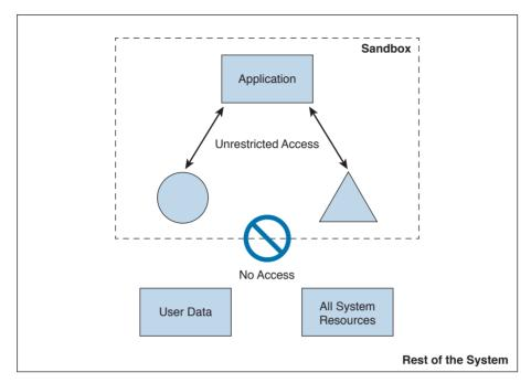
Figure 10-2 Example with a Sandbox
