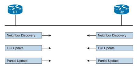
Figure 1-60 Example of EIGRP Message Exchange
