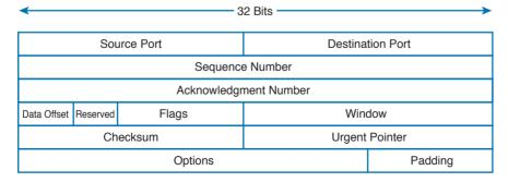
Figure 1-81 TCP Header Structure
