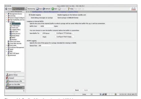
Figure 11-2 Enabling Logging via ASDM
