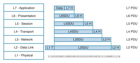
Figure 1-7 Encapsulation in the OSI Model
