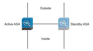
**Figure 2-6** Firewalls in Active-Standby Failover Mode
