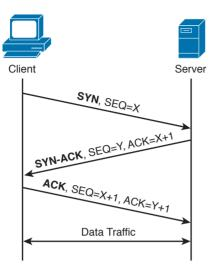
Figure 1-82 TCP Three-way Handshake
