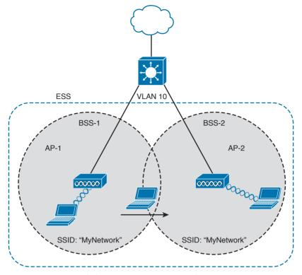
Figure 1-37 Extended Service Set (ESS) Example
