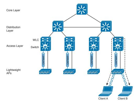
Figure 1-41 Converged WLC Architecture
