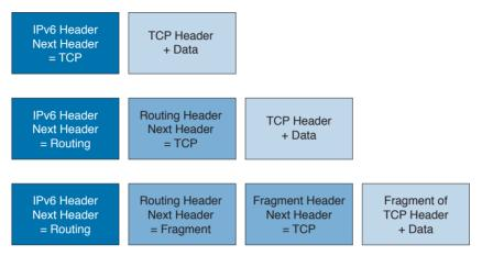
Figure 1-68 Chained Extension Header
