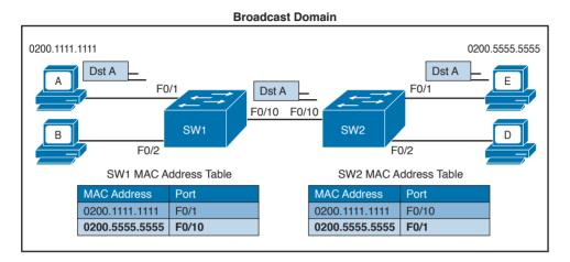
**Figure 1-23** Frame Forwarding and MAC Address Table Updates with Multiple Switches. Host E replies to a frame sent by Host A.
