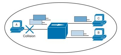
Figure 1-14 Collision Domain with a Hub or Repeater
