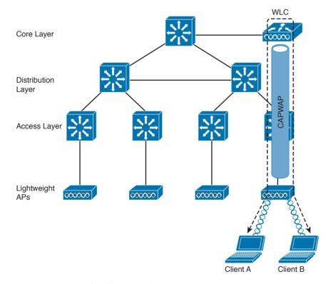
Figure 1-40 Centralized WLC Architecture
