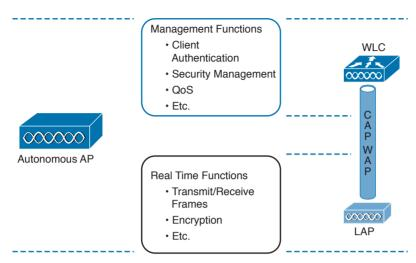
Figure 1-39 Comparison Between an Autonomous Access Point and a Lightweight Access Point
