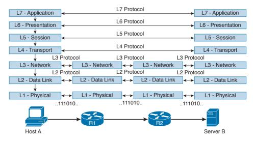
Figure 1-8 Flow of Information Through a Network Implementing the OSI Model In the rest of this book, we will use the OSI model and TCP/IP model layer names interchangeably.
