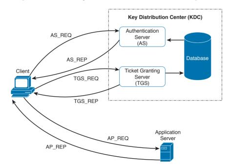
**Figure 5-7** Authentication and Authorization Using Kerberos
