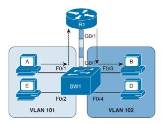
**Figure 1-32** *Router on a Stick (ROAS)*
