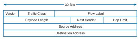
Figure 1-67 IPv6 Header
