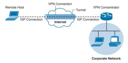
Figure 14-2 Remote-Access VPN Example
