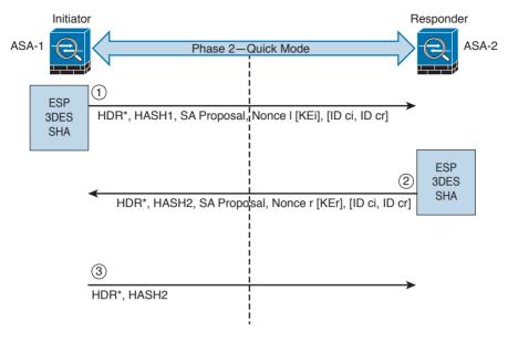
Figure 7-4 IPsec Phase 2 Negotiation
