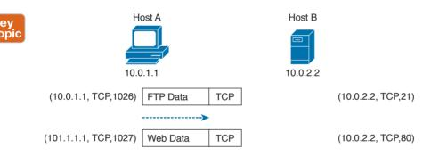
Figure 1-79 Example of TCP Multiplexing
