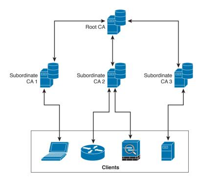
Figure 6-10 Hierarchical CA Deployment with Subordinate CAs
