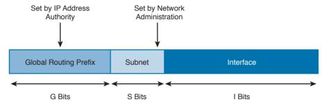
Figure 1-70 Global Unicast IPv6 Address
