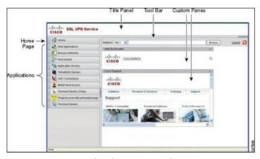
Figure 14-4 Cisco Clientless VPN Portal
