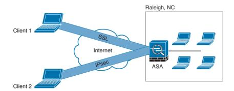
Figure 7-2 Remote-Access VPN Example
