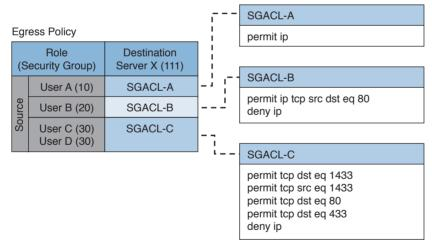
Figure 4-20 SGACL Deployment
