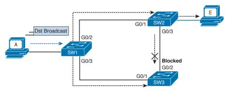
**Figure 1-25** Example of Layer 2 with STP Enabled
