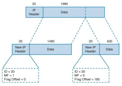
**Figure 1-45** Example of IPv4 Fragmentation
