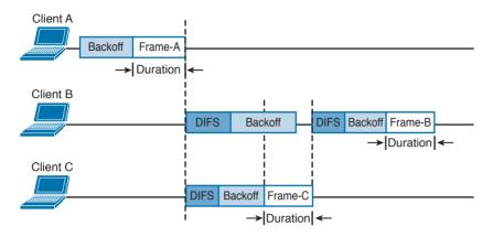
**Figure 1-34** *Transmitting Frames in a WLAN*
