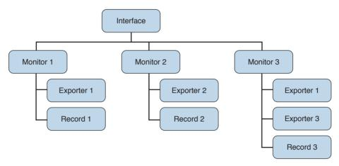
Figure 11-23 Flexible NetFlow Model
