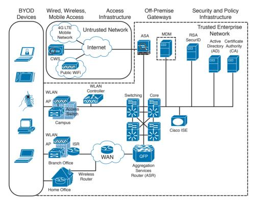
Figure 5-14 BYOD Infrastructure with an On-Premises MDM Solution
