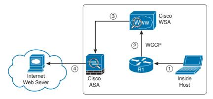
Figure 2-16 WSA Transparent Proxy Configuration
