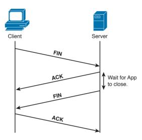
Figure 1-83 TCP Connection Termination
