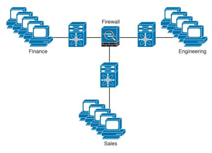
Figure 2-5 Firewall Providing Network Segmentation
