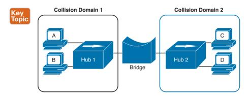
Figure 1-15 A Bridge Creating Two Collision Domains
