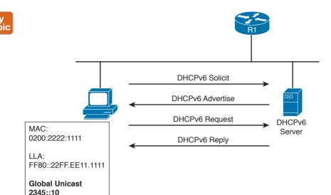
Figure 1-77 Stateful DHCPv6 Exchange for IPv6 Address Assignment
