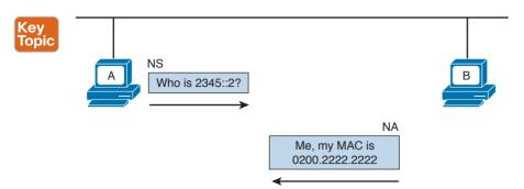
Figure 1-75 NS/NA Exchange to Get Link-Layer Address Information
