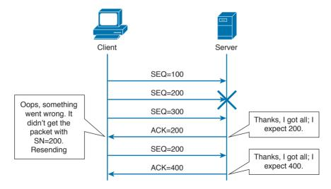
**Figure 1-85** *TCP Error Detection and Recovery*
