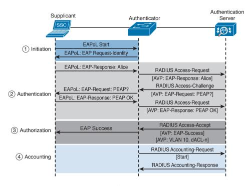
Figure 4-19 802.1x Port Access Control Exchange
