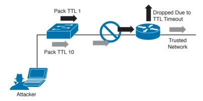
Figure 14-9 TTL Manipulation Attack
