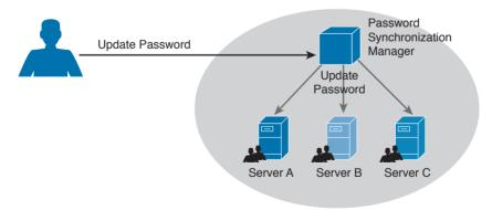
**Figure 5-2** *Password Synchronization System*
