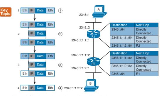
Figure 1-66 Communication Between Hosts Using IPv6
