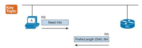
Figure 1-74 RS/RA Exchange
