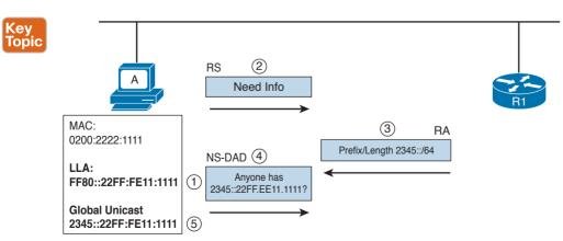
Figure 1-76 Address Assignment via SLAAC
