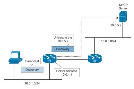
Figure 1-54 Example of DHCP Relay
