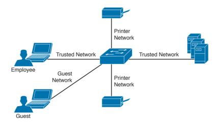
**Figure 14-11** *Example of Segmentation*
