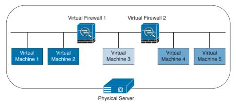
Figure 2-11 Virtual Firewalls Example
